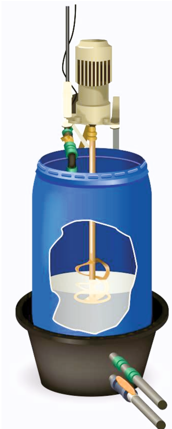
Band clamp lid barrel with stirring motor and water-cooling system on the bottom
