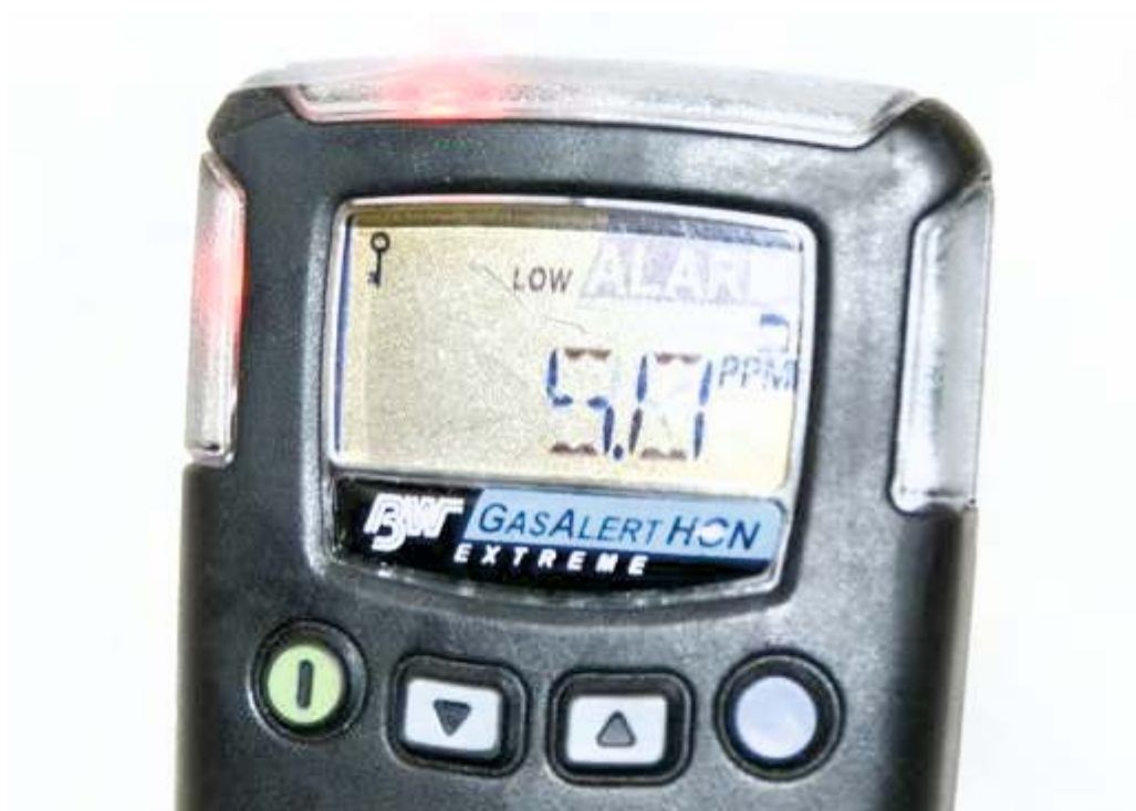
HCN measurement with the GasAlert
