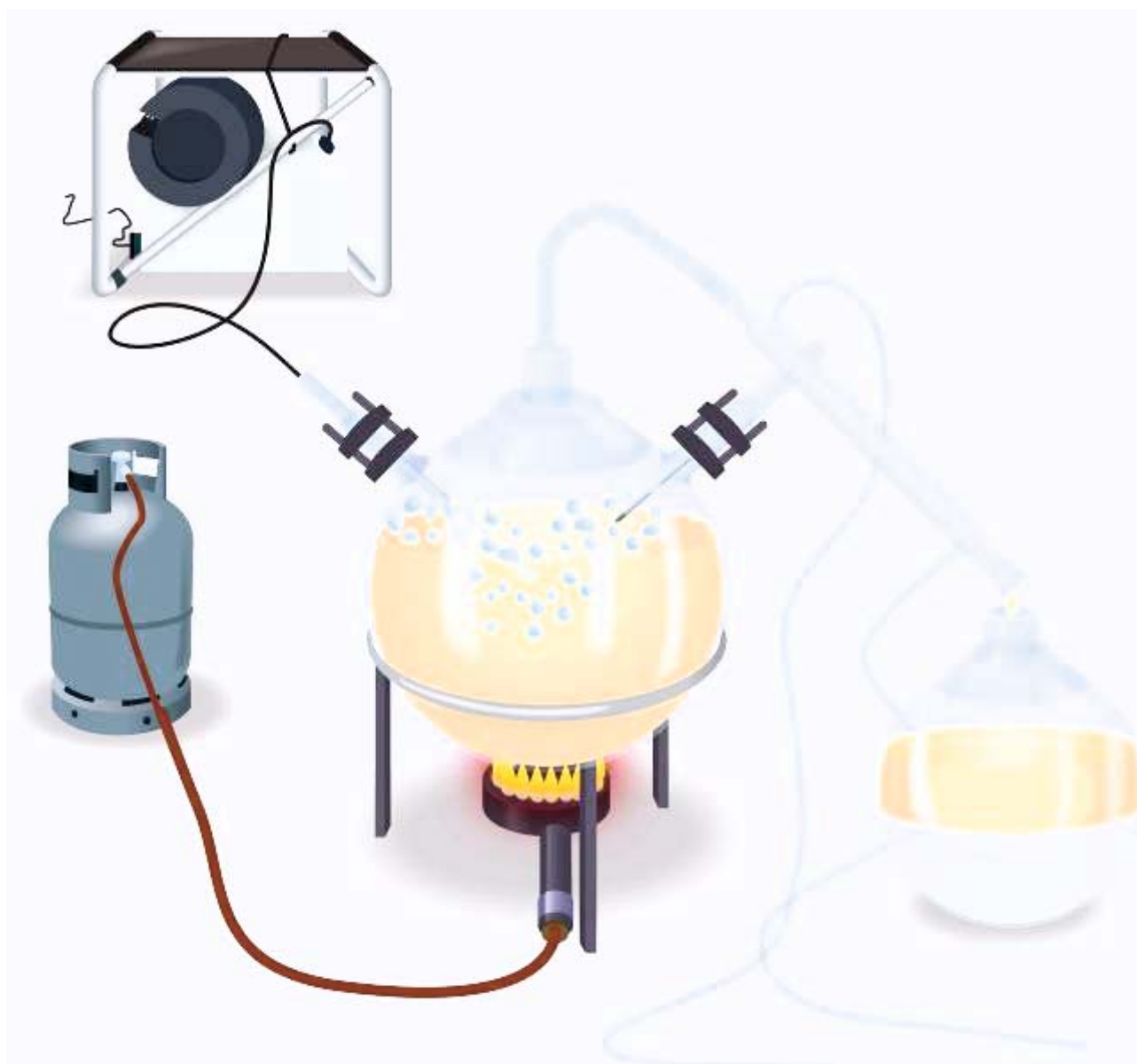
Schematic representation of steam distillation
