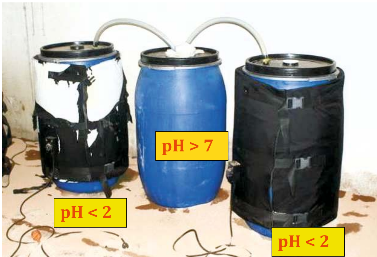
Conversion set-up with two reaction vessels and a gas scrubber in the middle.
