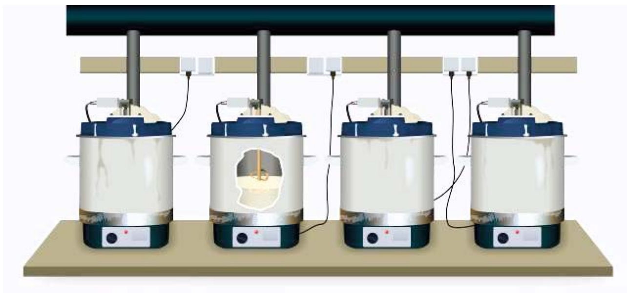
4 preserving kettles with joint exhaust installation
