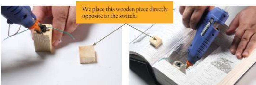
Fix the push switch on the wooden piece using glue.
