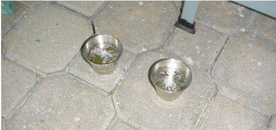
Ingots in their "molds" after pouring and solidifying, moved to the ground and left to cool.
