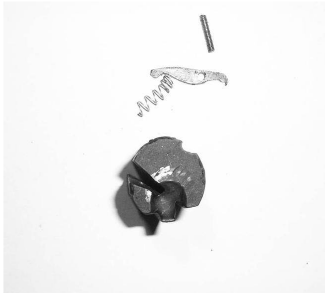
Inert dummy example containing no firing pin
