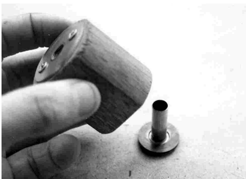
Insert the die over the case.
