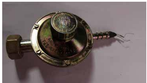
Ignition lamp in modified regulator.
