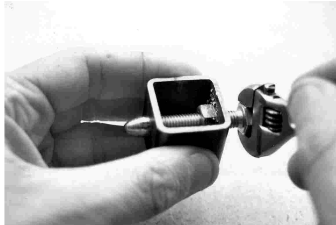
Press the bullet through the die.
