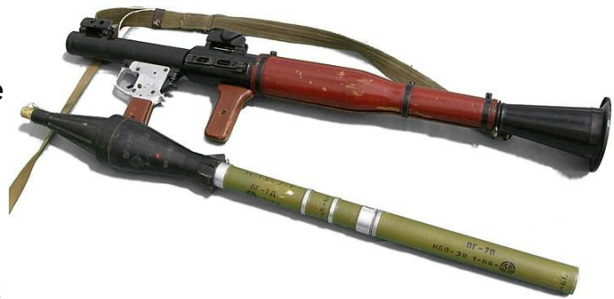
An RPG-7 launcher (top) with a Bulgarian PG-7G inert training An RPG-7 launcher (top) An RPG-7 launcher (top) with a Bulgarian PG-7G inert training warhead and booster (bottom).
