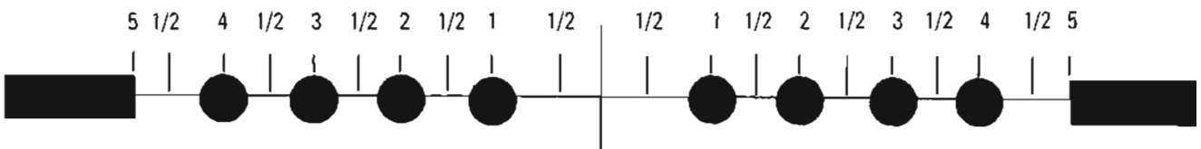
Wind compensation and moving target leads use the horizontal mil scale.
