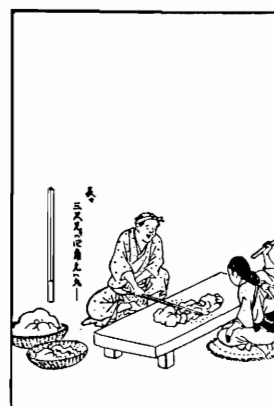
Papermaking. Series of Chinese woodcuts illustrating final steps of papermaking, from boiling the bark in lye, to washing, beating, drying, trimming, and packing the finished paper. From Kamisuki Chohoki's 18th century A Handy Guide to Papermaking.
