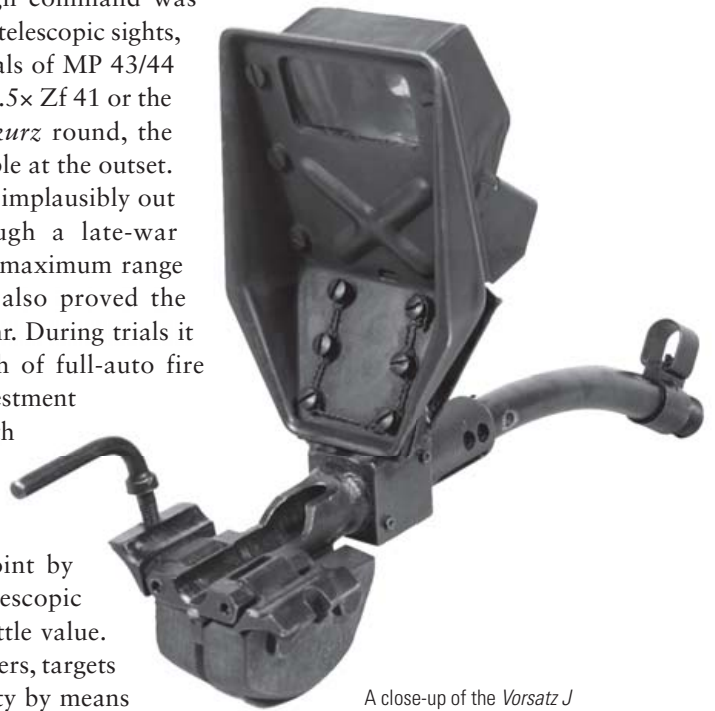
A close-up of the Vorsatz J device, showing the prismatic aiming device from the rear. Once fitted to an StG 44, the Vorsatz J fundamentally unbalanced the weapon, and critically weakened the barrel after firing a few hundred rounds. (Cody Images)
