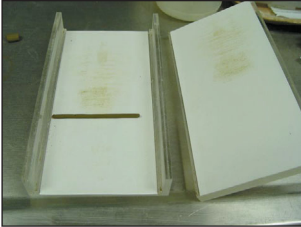
FIGURE 3 Rolling moist soil into a thread. (Photo courtesy of the Geotechnical Laboratory of the University of Texas at Arlington)
