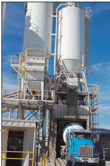
FIGURE 21.22 A truck mixer being charged with the mix. The control room is located adjacent to the charging station to allow the technician to observe and control the process. The control room has glazed openings toward the charging station; see Figure 21.23.
