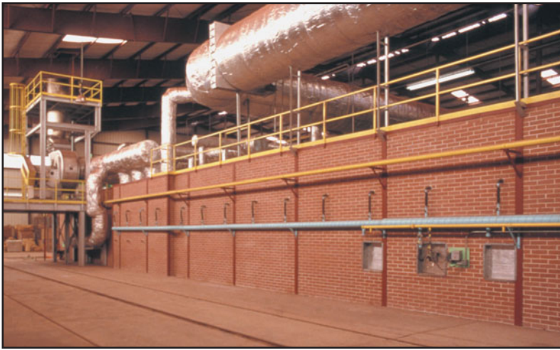
FIGURE 24.14 A typical tunnel kiln. (Photo courtesy of Acme Brick Company, Fort Worth, Texas)
