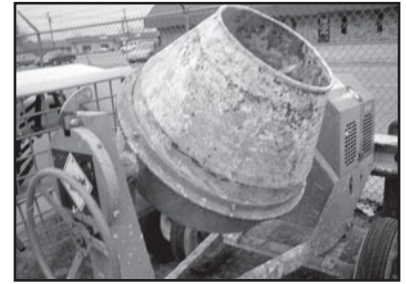
FIGURE 21.19 A transportable mixer for on-site mixing of small quantities of concrete.
