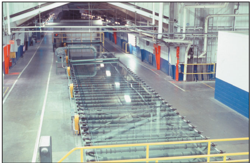
FIGURE 30.6 In the float glass manufacturing process, glass emerges as an endless ribbon at room temperature. (Photo courtesy of PPG Industries Inc.)
