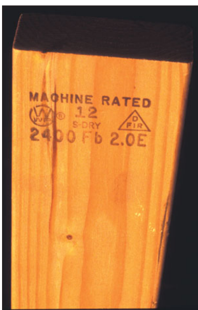
FIGURE 13.41 A typical grade stamp on a machine stress-rated (MSR) lumber.
