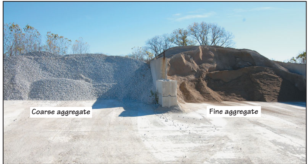
FIGURE 21.21 Stockpiles of coarse and fine aggregates in a concrete ready-mix plant. Observe the separation between different aggregates to ensure correct proportioning of the mix.
