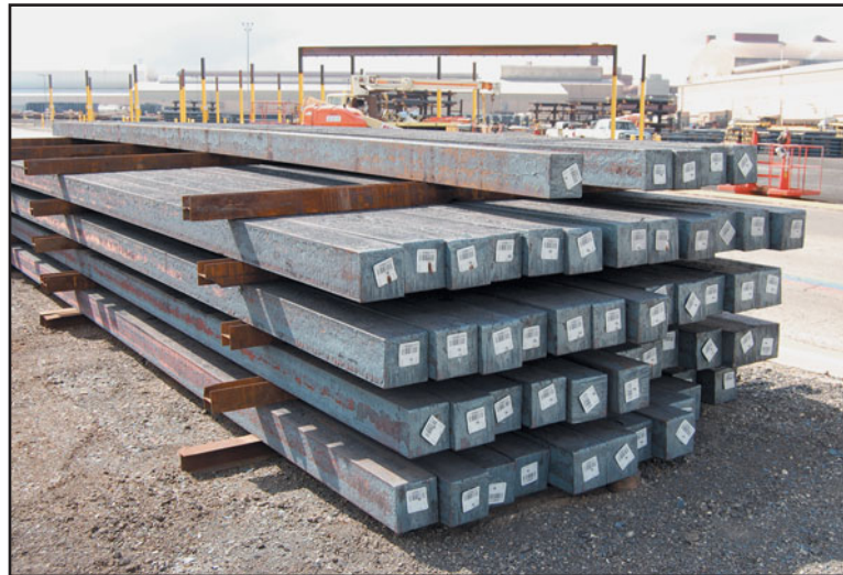
FIGURE 18.7 Rectangular billets used for rolling into channels, angles, bars, and rods.
