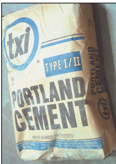
FIGURE 21.9 Type I/II portland cement. A portland cement bag (1 ft 3 ) generally weighs 94 lb.
