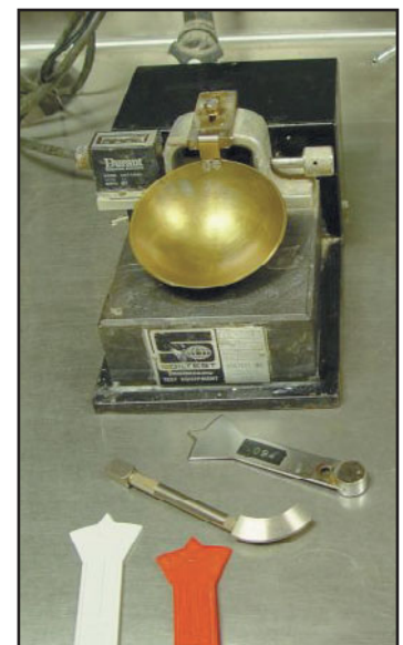
FIGURE 2 A liquid limit testing apparatus. (Photo courtesy of the Geotechnical Laboratory of the University of Texas at Arlington)
