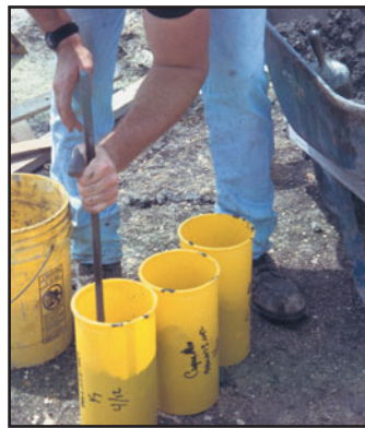
FIGURE 21.17 Casting of concrete test cylinders.
