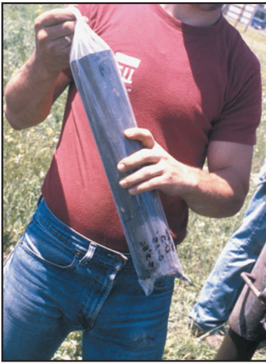
FIGURE 11.3 Soil samples obtained from borings through the use of a sampling tube are wrapped in plastic, labeled with the date of sampling, location of boring at the site, depth, and so on, and sent to a geotechnical laboratory.
