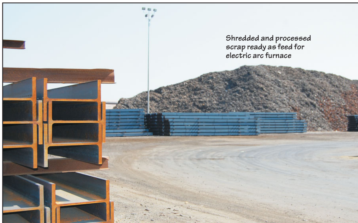
FIGURE 18.10 A view of the yard of the Gerdau Ameristeel Plant in Midlothian, Texas, showing the shredded ferrous scrap in the background and finished steel sections in the foreground.
