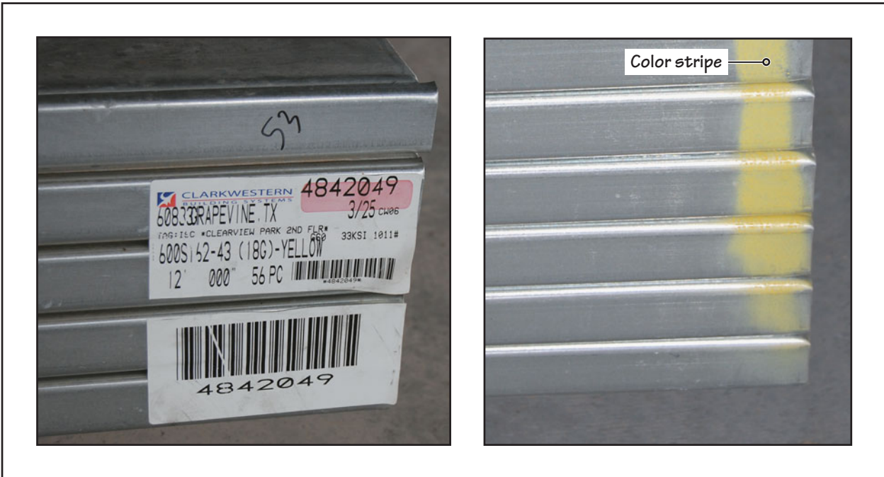
FIGURE 20.2 Cold-formed steel members carry a label on the strapped bundle that identifies their cross-sectional dimensions and sheet thickness. Additionally, members that are 33 mil and thicker, carry a color stripe that identifies the member's gauge number (sheet thickness) as per ASTM Standard C955
