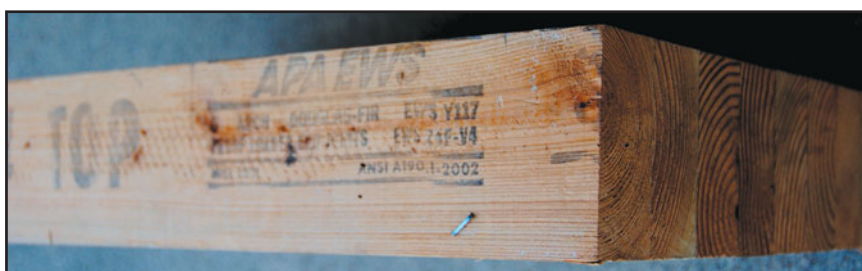
FIGURE 14.7 An unbalanced glulam beam showing the beam's top face.
