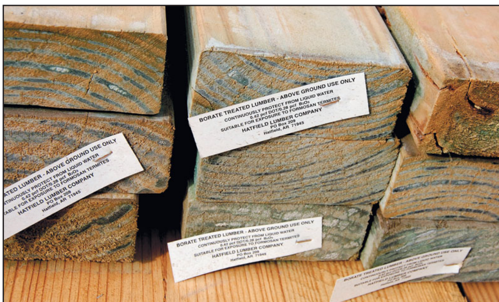
FIGURE 13.46 A pressure-treated lumber pile with end tags.
