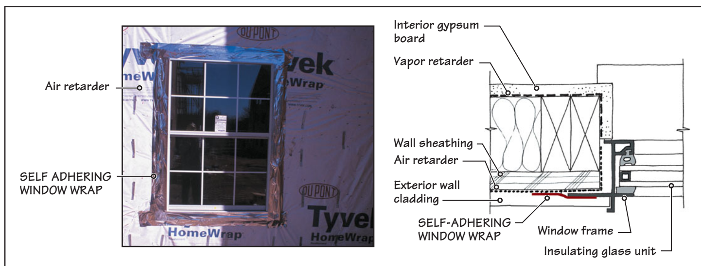
FIGURE 6.6 A self-adhering tape on the outside of a window (referred to as window wrap ) to reduce air leakage through the joint between the window and the wall, photographed before the application of exterior cladding.
