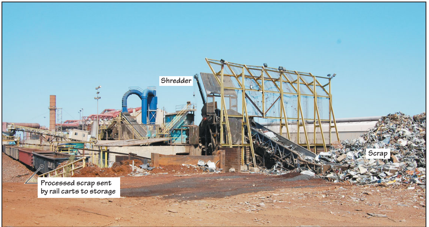
FIGURE 18.9 A scrap shredder in the Gerdau Ameristeel Plant in Midlothian, Texas. After the scrap is shredded, it is separated into ferrous and nonferrous parts through magnetic separation. The ferrous scrap is then sent by rail carts to storage, ready for feed into the electric arc furnace; see Figure 18.10.
