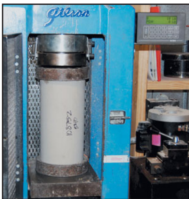
FIGURE 21.18 A concrete test cylinder in position in the testing machine, ready to be compressed to failure (see also Figure 4.6).
