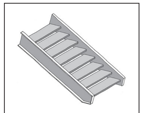
FIGURE 35.3 A stair with open risers.
