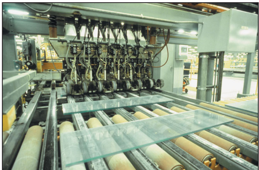
FIGURE 30.7 Glass is cut by automatic cutters to the required sizes before packing and shipping. (Photo courtesy of PPG Industries Inc.)
