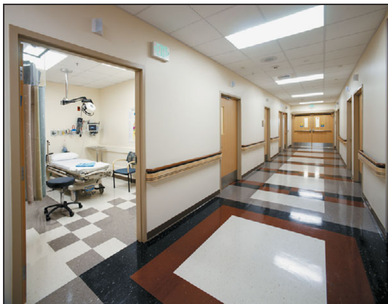
FIGURE 36.14 A multicolored pattern of vinyl composition tiles installed in a hospital. (Photo courtesy of HKS Inc.)
