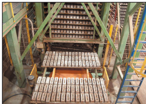
FIGURE 24.17 Several hundred bricks are molded in one single pass in the molding machine. (Photo courtesy of Acme Brick Company, Elgin, Texas)
