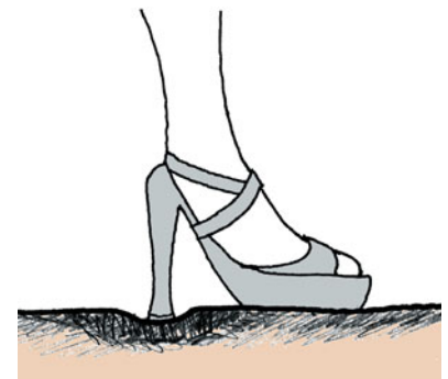
Local crushing or settlement (bearing failure)
