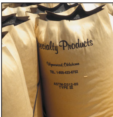
FIGURE 33.9 Types III and IV asphalt are available in paper-wrapped kegs, as shown.
