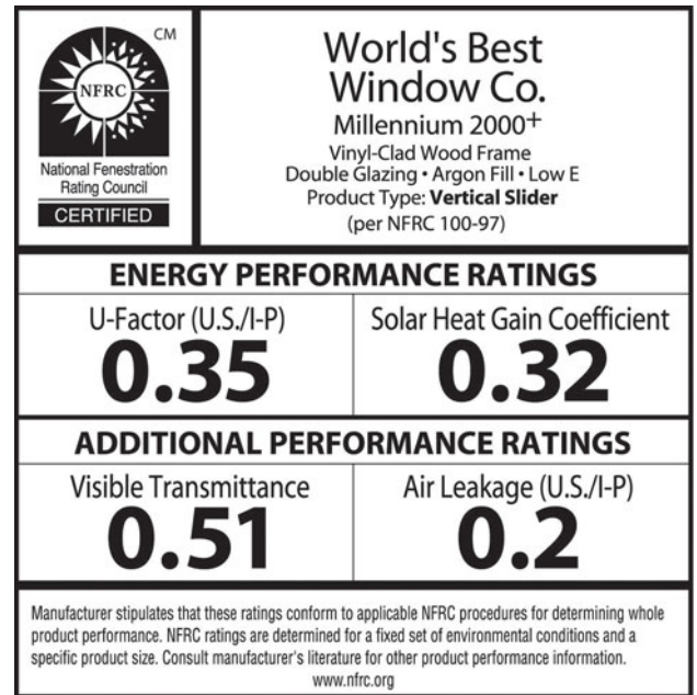
FIGURE 31.6 A typical label on an NFRC-rated window; see also Figure 31.9(a). (Illustration courtesy of National Fenestration Rating Council)
