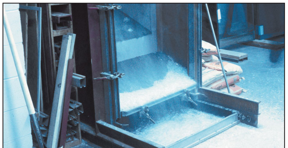
(b) Glass after the test. The size of broken glass pieces (which must be small enough and within the limits specified in the test standard) indicate that the glass has passed the test.
