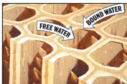
FIGURE 13.23 Free water and bound water in wood cells. (Photo courtesy of Southern Forest Products Association)
