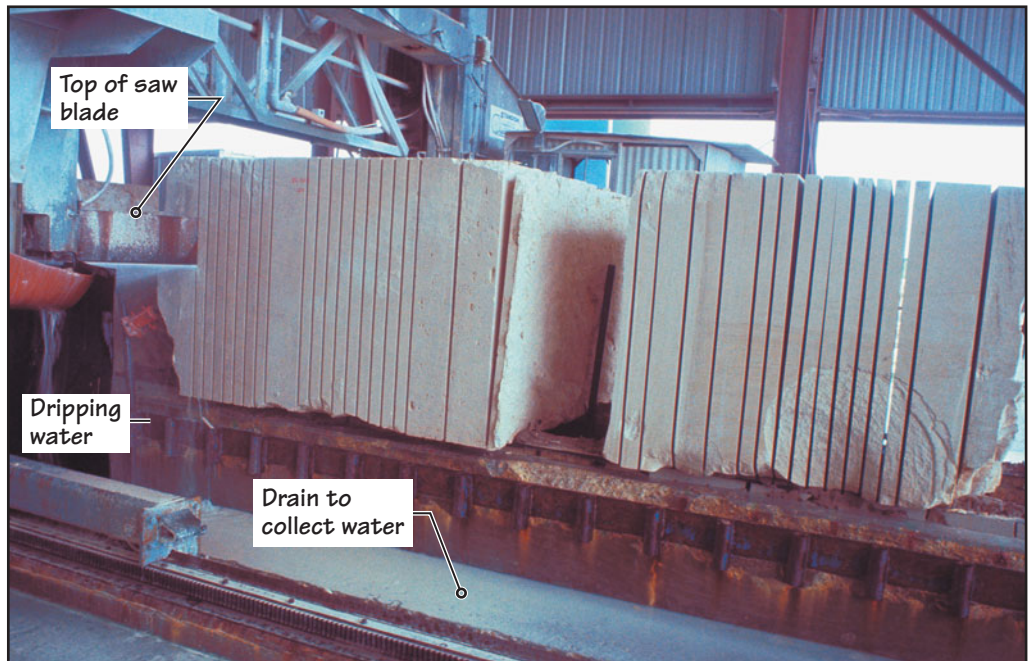
FIGURE 25.30 Conversion from stone blocks to slabs through sawing. Note that the sawing operation needs a great deal of water to cool the blade. Photo taken at Texas Quarries, Austin, Texas.
