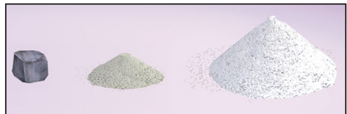
FIGURE 6 Three stages of perlite production show the great increase in volume that takes place on expansion by heating of the perlite rock. Although this illustration refers to perlite rock, it applies to all rocks that contain some water and are commonly used in expanded state (see Figure 21.14).
