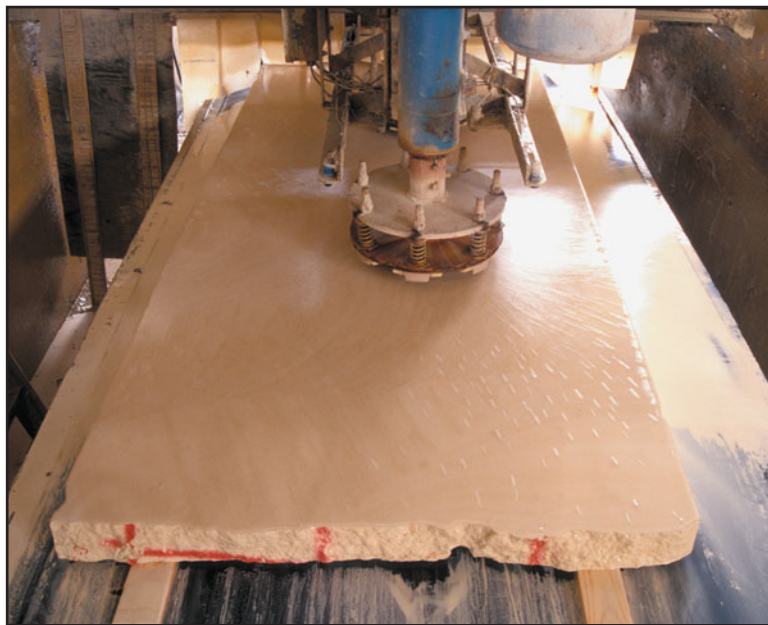
FIGURE 25.32 Honing (grinding) of stone slabs using water to cool the grinders. Photo taken at Texas Quarries, Austin, Texas.
