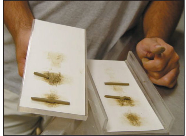
FIGURE 4 As the moist soil thread is progressively dried while rolling, it breaks. (Photo courtesy of the Geotechnical Laboratory of the University of Texas at Arlington)
