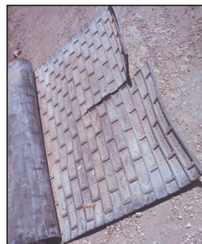
FIGURE 28.47 A rubber template form liner used with thin brick-faced panels.
