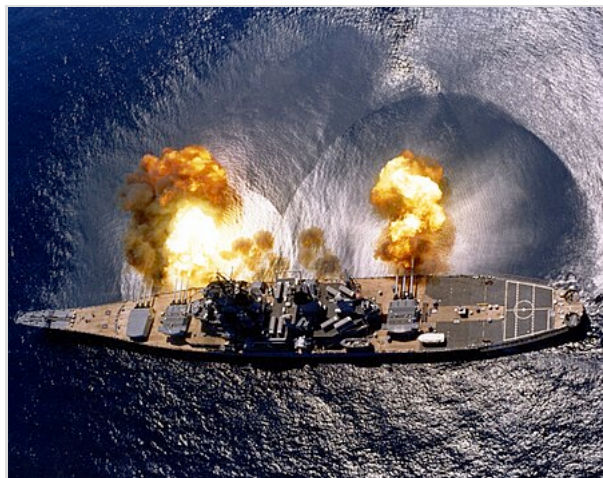
USS Iowa fires a broadside of nine 16"/50 and six 5"/38 guns during an exercise
