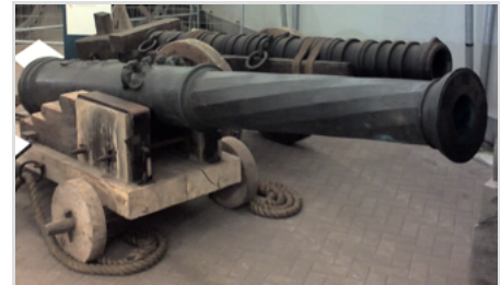
A cast bronze culverin (front) and a wrought iron port piece (back), modern reproductions of two of the guns that were on board the Mary Rose when she sank, on display at Fort Nelson near Portsmouth
