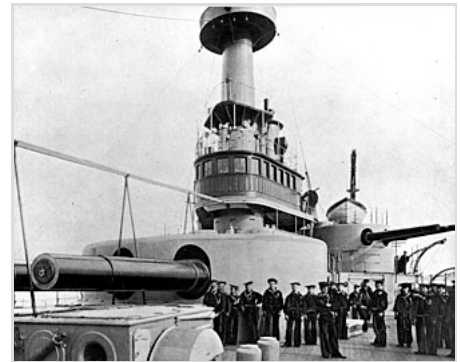
USS Indiana , an example of the intermediate battery principle with its forward 13-inch and forward port 8-inch gun turrets
