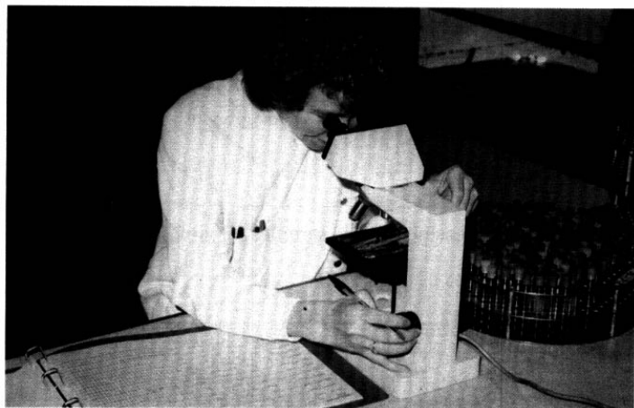
Figure 1. Each tube on the roller (seen on the right of the microscope) is examined under low power for evidence of a cytopathic effect.
