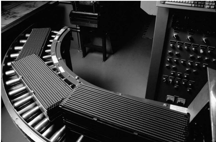
FIGURE 12.7 Stacks of completed nuclear fuel pellets being moved in a fuel fabrication facility.
