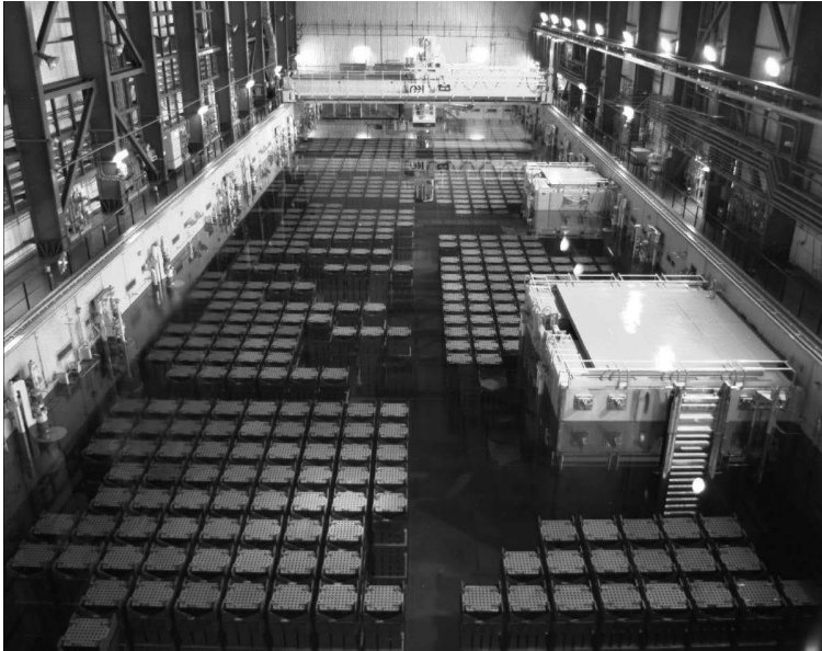
FIGURE 14.13 Storage of spent fuel in pool, La Hague France. (Courtesy of AREVA.)
