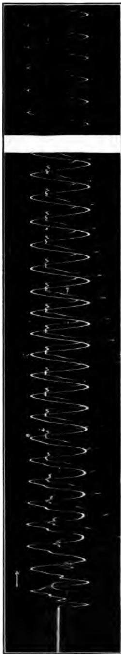
Fig. 30. — cp10075. — Transient Starting Current of Alternating-current Transformer. 20 Cycles Later.
