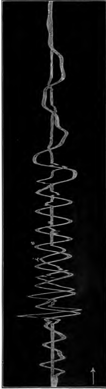
Fig. 48B. — cd10049. — Oscillogram of High-frequency Oscillation Preceding Low-frequency Oscillation of Compound Circuit Caused by Switching 154 miles of 100,000 Volts Transmission Line and Step-down Transformer off another 154 Miles of 100,000 Volts Line; High-tension Switching.
