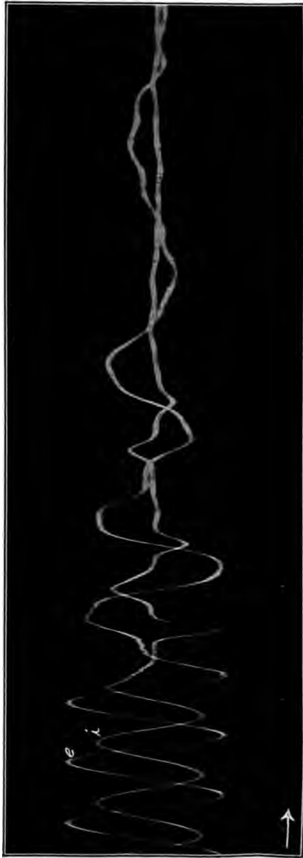
Fig. 41. — cd10045 . — Oscillogram of Compound Circuit of 154 Miles 100,000-volt Transmission Line and High-tension Coils of 10,000-kw. Step-up Transformers, Switching off by Low-tension Switches. High-tension Current and Low-tension Voltage.
