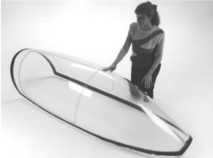
Figure 2. Concept for explosive fracture of F-16 aircraft canopy to allow through-canopy ejection.
