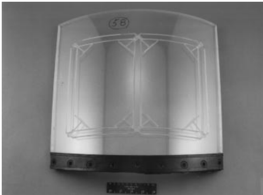
Figure 5. View of grooves in mini-panel. The parallel grooves will contain explosive cord. The "T" grooves and circular cavities will contain data sheet.
