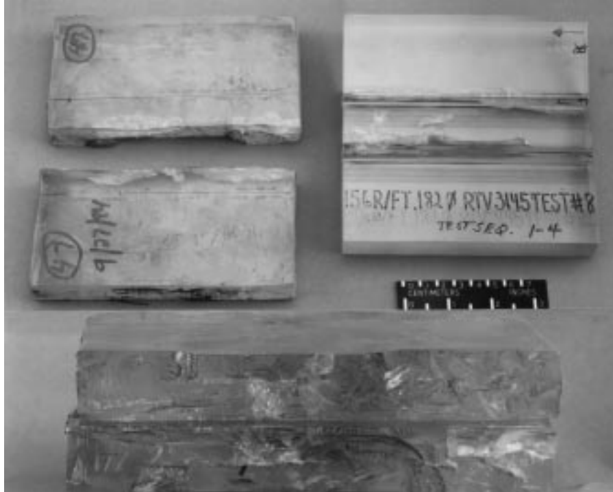
Figure 11. Results of explosive fracturing tests on 0.875-inch polycarbonate. The explosive cord was embedded in the plate on the right and in the trilaminar test at the left. The bottom photograph is an edge view of the results of the trilaminar test.
