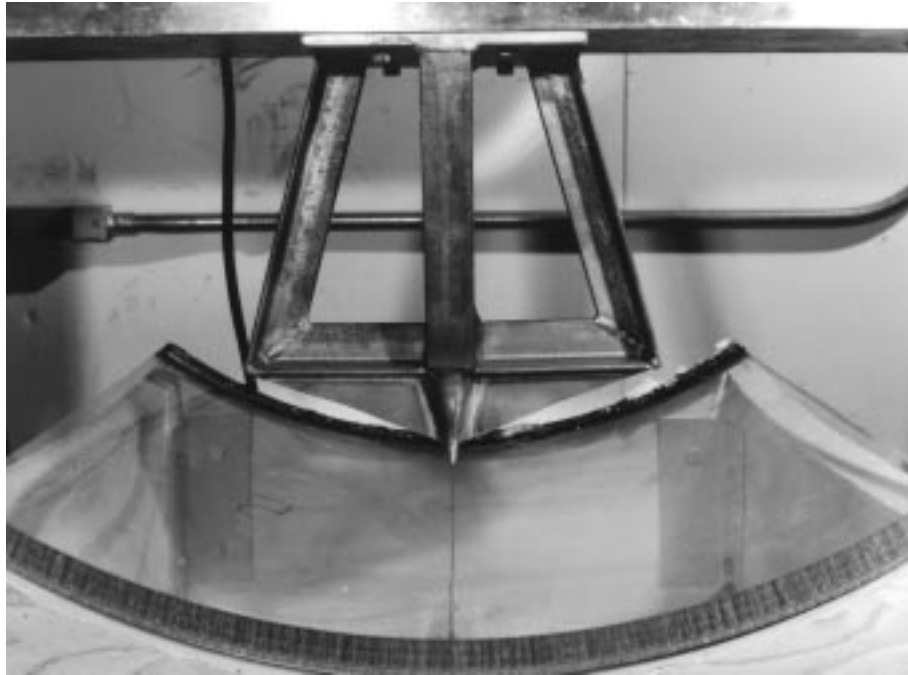
Figure 4. Mockup of seat headrest interface used in push-out tests to split and force open fractured canopy.
