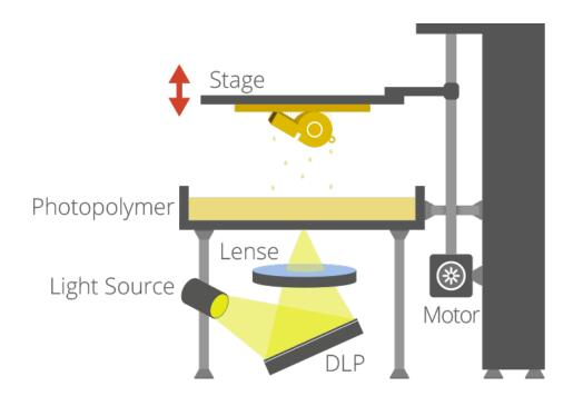
DLP — or digital light processing — is a similar process to stereolithography in that it is a 3D printing process that works with photopolymers. The major difference is the light source. DLP uses a more conventional light source, such as an arc lamp, with a liquid crystal display panel or a deformable mirror device (DMD), which is applied to the entire surface of the vat of photopolymer resin in a single pass, generally making it faster than SL.
