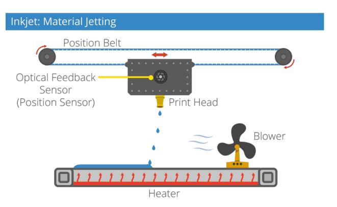
**Material jetting:** a 3D printing process whereby the actual build materials (in liquid or molten state) are selectively jetted through multiple jet heads (with others simultaneously jetting support materials). However, the materials tend to be liquid photopolymers, which are cured with a pass of UV light as each layer is deposited.
