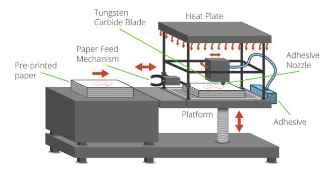
SDL is a proprietary 3D printing process developed and manufactured by Mcor Technologies. There is a temptation to compare this process with the Laminated Object Manufacturing (LOM) process developed by Helisys in the 1990's due to similarities in layering and shaping paper to form the final part. However, that is where any similarity ends.
