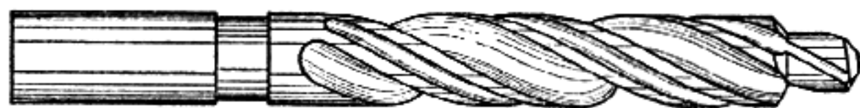
Standard commercial three groove twist drill, with pilot ground on it, to drill out old barrels for relining.
