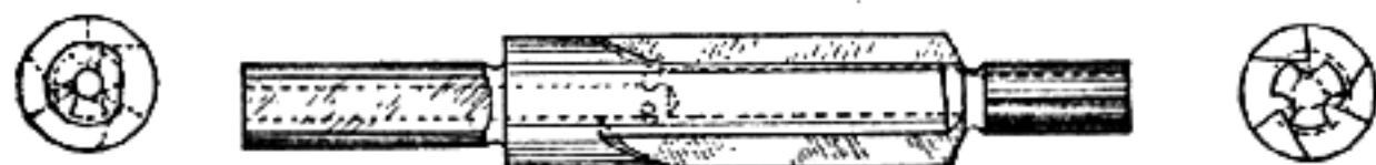
Three groove drill of high speed steel, with straight grooves, to bore out old barrels for relining.
