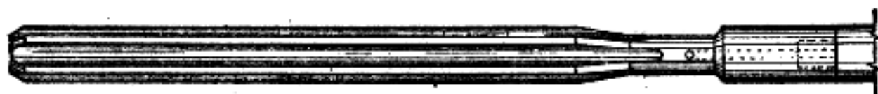
Six-groove barrel reamer, of the type commonly used in sets of three, in graduated sizes.
