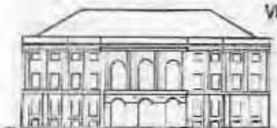
THICK WALLS DEEPLY RECESSED WINDOWS
